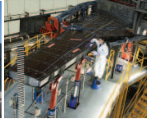
Bombardier CSeries Wing Test
